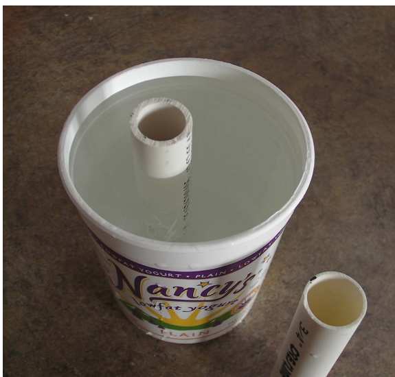
Figure 1 (above): two PVC tubes, the thicker Schedule 40 tube is shown floating in water. Its bottom is taped closed with clear packing tape, and it is weighed down with pennies as simulated batteries. The thinner "Type 2" PVC tube is shown outside of the yogurt tub.
